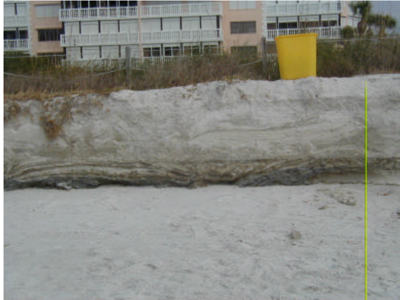
Figure 2: Photograph of oily, cohesive band of material found at Location LK 4. This picture was taken January 15, 2004.
